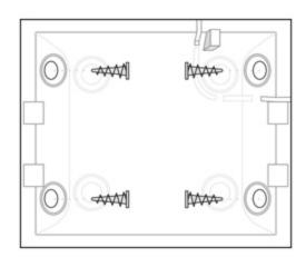
1. Attach the SmartBracket panel to the surface using bundled screws, using at least two fixing points (one of them — above the tamper). After selecting other attachment screws, make sure that they do not damage or deform the panel.
